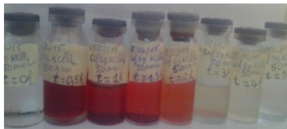
Fig. 7 Photo of the solution withdrawn from the wastewater tank during electrolysis (from left to right : t = 0 h; 0.5 h; 1 h; 1.5 h; 2 h; 3 h; 4 h; 5 h)
